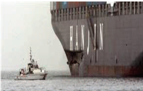
Damage to the Cosco Busan after colliding with the Bay Bridge.
